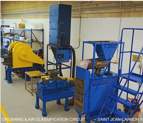
*Image 3: Crushing & Air Classification Circuit*
