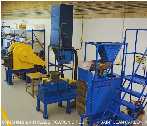
Image 3: Crushing & Air Classification Circuit
