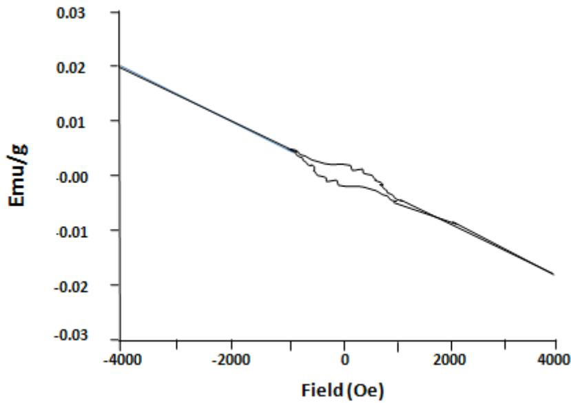
**Chart 2** Shows ferromagnetic properties. Saturation magnetism is 0.11emu/g coercivity is 173Oe
