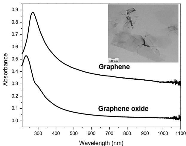
Fig. 1: UV-Vis spectra of graphene oxide and graphene. The small inset is the TEM micrograph of the graphene sheets.
