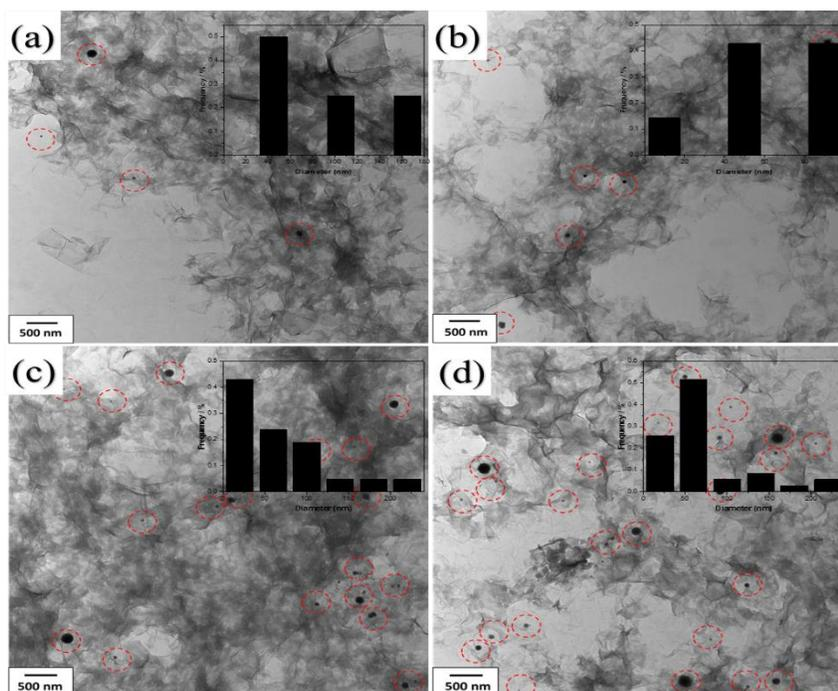
Fig. 3: TEM micrograph of the YBCO particles on the surface of the substrate under different deposition time ( $t$ ) (a)  $t = 0.5$  hr; (b)  $t = 1.0$  hr; (c)  $t = 1.5$  hr; (d)  $t = 2.0$  hr; (e) TEM-EDX spectrum of the graphene/YBCO hybrid nanosheets ( $t = 2.0$  hr).
