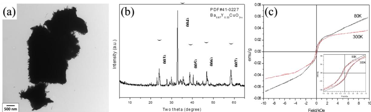
Fig. 2: (a) TEM micrograph of YBCO particles used as the precursor of YBCO nanoparticles produced by MAPLE. (b) XRD profile of the YBCO powder, similar with the XRD profiles of  $\text{Ba}_{0.68}\text{Y}_{0.33}\text{CuO}_{3-x}$  (PDF#41-0227). (c) Hysteresis loops of YBCO powder at 300 K and 80K.
